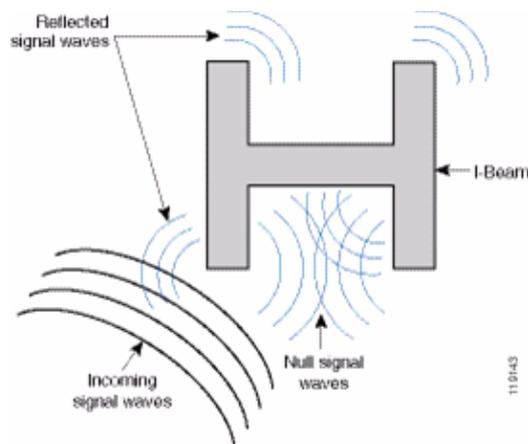
The access point and antenna placement in Figure 19 is better because it is away from the I-beams and there are fewer reflected signals, fewer null points, and less multipath interference. This placement is still not perfect because the Ethernet cable should not be coiled up so close to the antenna. Also, the access point could be turned with the 2.4GHz antennas pointed to the floor. This provides better coverage directly below the access point. There are no users above the access point.
