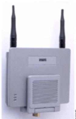
Figure 24 shows the Cisco Aironet 2012 diversity patch antenna mounted to a wall. In this case, the Cisco AP1200 is mounted above the ceiling tile.
