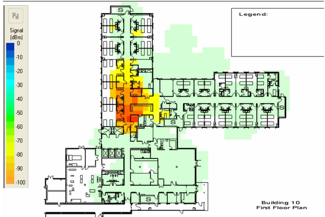
Figure 3-2 AirMagnet Co-Channel Interference Possibility Example
